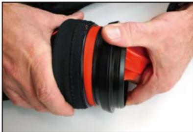
**7.** Push together with both hands on all sides until you hear a clicking sound and/or see the edge of the suit is close to the suit ring on all sides. Check the Silicone is in place and not wrinkled.
