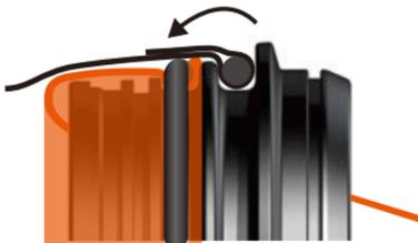
**5.** Pull the drysuit Neoprene cuff to cover the seals, leaving a gap of approximately 4mm and mount the cover ring as shown.
