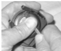
Fig. 125 - BATTERY HATCH REMOVAL (Tool)
