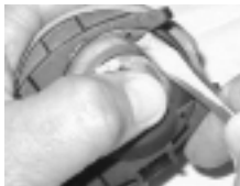
Fig. 130 - TIGHTENING VT3 HATCH RING
