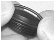
Fig. 131 - TRANSMITTER O-RING INSTALLATION
