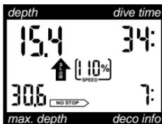
Optimal ascent rate varies depending on depth between 7 and 20 m/min. It is displayed in percent of the reference variable. If the ascent rate is greater than 100% of the set value, the black arrow <SLOW> appears. If the ascent rate exceeds 140%, the arrow starts flashing.
