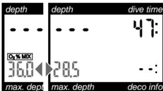
After reaching the surface, Aladin® Pro Ultra switches into wait-mode automatically for five minutes. This is the time span necessary to recognize the end of the dive.
