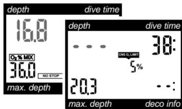
Current depth is given in 10 cm-increments. On switching on and at a diving depth of less than 0.5 metres the void display <---> appears.
