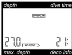
1. From ready-mode, you switch into the diveplan input stage by twice bridging contacts B and -.
