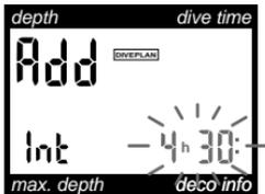
1. From surface-mode, you switch into the diveplan input stage by twice bridging B and –.
