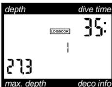
1. The logbook is selected by bridging contacts B and + in ready- or surface-mode. Indication **LOGBOOK** appears. If Aladin® Pro Ultra has been in surface-mode before, the surface interval appears as well. You go back into ready- or surface-mode by B and -.
