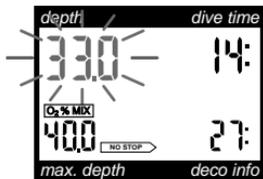
The tolerable partial pressure of oxygen can be set by means of a MemoMouse and the DataTalk software to between 1.2 and 1.95 bar (see page 76). The set value and the information about the actual ppO<sub>2</sub> are not displayed.
