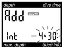
Presetting the surface interval (only during desaturation)
