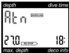
The Aladin® Pro Ultra calculates according to the planned surface interval the expected production of microbubbles. The diver should increase the surface interval if <Atn> (Attention) is displayed. This will reduce the risk of micro bubble production in the pulmonary system.
