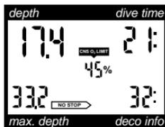
Oxygen toxicity is calculated on line as a function of depth values and the gas mixture. The toxicity is displayed in 5% increments as a percentage of the maximum value tolerated (O<sub>2</sub> clock), together with the symbol <CNS O<sub>2</sub> LIMIT>. This display is in the same place as the ascent rate display.
