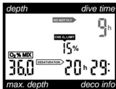
The waiting period until the next flight is indicated as follows: **DO NOT FLY**. Beside this the time in hours that should pass before a flight is displayed.
