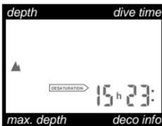
Aladin® Pro Ultra measures the atmospheric pressure even while in sleep-mode. If the computer detects a higher altitude, it switches into surface-mode automatically. Desaturation time indicated at this moment refers to adaptation time at this altitude. If diving starts within this adaptation time, Aladin® Pro Ultra treats it as a repetitive dive, since the body still has a higher saturation.
