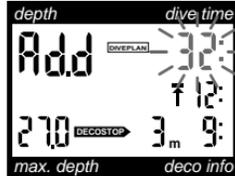
1. In order to plan a dive that requires decompression, wait until the scrolling no-stop time shows the desired depth.
