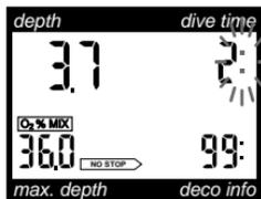
The whole time spent below a depth of 1.2 metres is displayed as dive time in minutes. While the dive time is running, the colon on the right of the figures is flashing in one second intervals. Maximum dive time displayed is 199 minutes.
