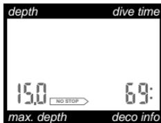
After confirming the surface interval (if possible), no-stop times are displayed in 3 metre-increments. The process starts with 9 metres. The no-stop time for every 3 metre-increment is displayed for about 3 seconds (scrolling no-stop times).
