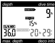
When **DESATURATION** appears, the Aladin® Pro Ultra is in surface-mode. Desaturation time in hours and minutes, the set mixture (percentage of oxygen) and, if available, oxygen toxicity is displayed next to it. Desaturation time is continually indicated until the next dive or until it reaches zero. The display is switched off to save energy three minutes after the last manipulation is made (surface-sleep-mode).
