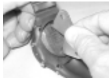
Fig. 144 - BATTERY HATCH REMOVAL (Tool)
