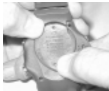
Fig. 145 - ALTERNATE HATCH REMOVAL
