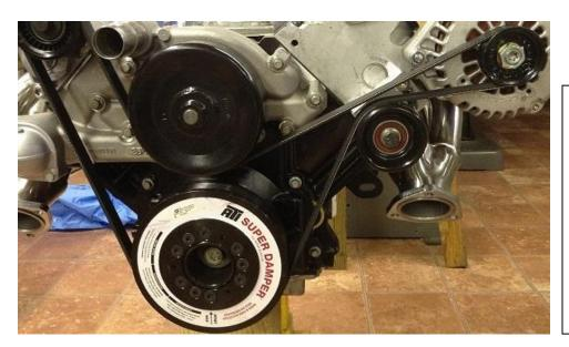
Using a 15mm socket, rotate factory tensioner clockwise to get the belt on. Use a 68.5" belt with stock diameter balancers and standard water pump.
