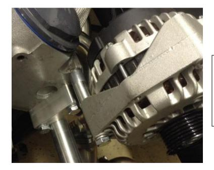
Using a 17mm socket, snug this bolt at location B so that alternator will hold in position, but still rotate. Do not tighten yet.
