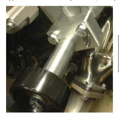
Install the round idler boss/spacers and pulley onto the idler block and tighten with a 17mm wrench. Do not over torque.
