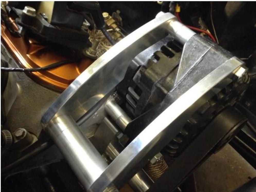
Insert the M10x120mm bolt through the first bracket and alternator. Then insert spacer(s) between alternator and second bracket. **Camaro uses the shortest**
