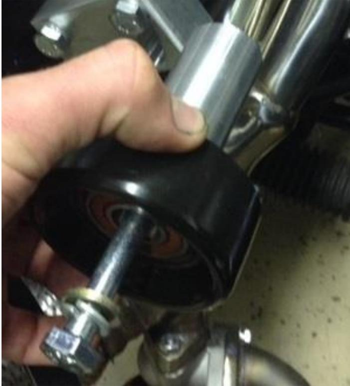
Slide the idler pulley on the aluminum boss.
