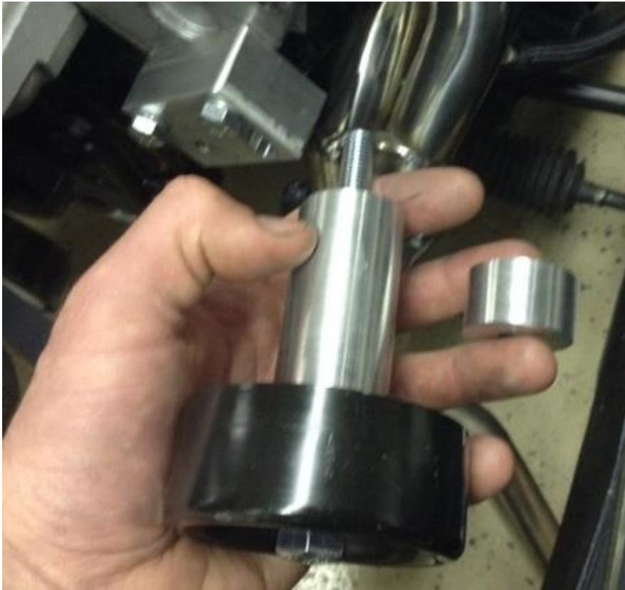
Use the supplied  $\frac{3}{4}$ " spacer only if using truck balancer.
