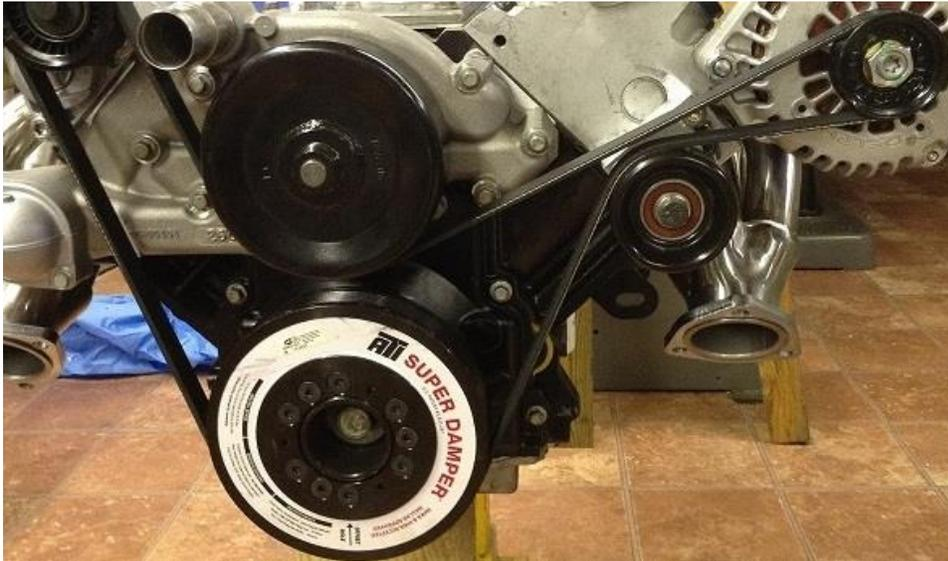
Using a 15mm socket, rotate tensioner clockwise to get belt on. Use a 68.5" belt with stock diameter balancers. 49" belt for electric water pump
