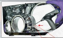
Here you will need to notch out a small section of the chrome piece in order for the halo to fit securely. Route the wires of this ring through the hole as well.
