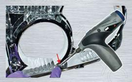
Once the chrome piece and the lens is seperated, drill a small hole here for the wires to be routed through.
