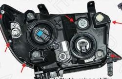
A) Start by using a phillips screwdriver and remove the 6 screws holding the lens and housing together.
