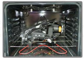
STEP #1: IN ORDER TO OPEN THE LIGHT WE WILL FIRST NEED TO HEAT THE HOUSING. IF USING A HEAT GUN BEGIN BY HEATING THE SEAL EVENLY WHILE CONSTANTLY MOVING THE HEAT GUN. IF USING AN OVEN: PREHEAT TO 225°F AND PLACE THE LIGHT IN THE OVEN FOR 10 MINUTES.
