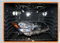
Remember to tighten down all 6 screws after you remove the headlight from the oven. While the easy seal is still heated, tightening the screws down will secure the easy seal together.
