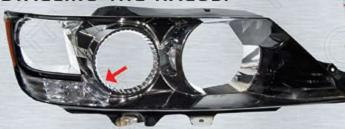
Now remove the black housing from the rest of the headlight. The bezel around the projector is where the halo will be mounted.
