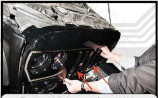
There is a pin in the center of the grill. Make sure that is lined up first, then apply pressure to the bottom of the grill to snap in place.
