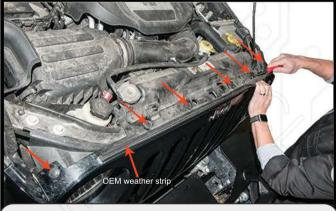
2 Use a flat head screwdriver or panel tool to remove the 6 clips holding the OEM grill in place.
