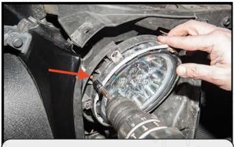
**5** Once the OEM grill is removed, use a T15 torx to remove the headlight adjuster.
