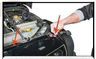
Once the Vector Grill snaps in place, re-install the clips on the top of the grill. Apply the rubber gasket across the top of the Grill and enjoy!
