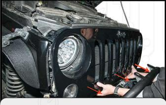
Start from the bottom and pull back on the OEM grill to release it from its fasteners.
