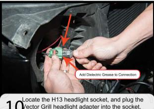
Vector Grill headlight adapter into the socket. Check your connector: https://bit.ly/2xaSeNN
