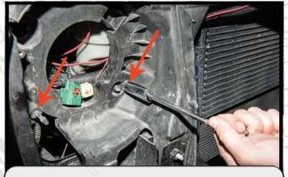
Use a 15mm Socket to remove the two headlight posts. Refer to picture above for the locations.
