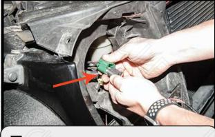
Unplug the OEM headlight adapter from the factory wiring harness.
