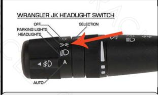
Now switch on the Parking Lights and CHECK b be sure the DRL Tuns on if not unplug Step 9 and revers the plug direction and test again.
