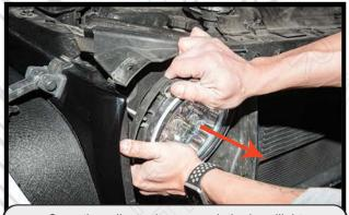
Once the adjuster is removed, the headlight and bracket can now be separated from the vehicle.
