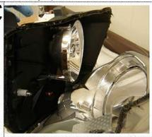
4) If the lens does not separate easily from the housing insert the lamp back into the oven for another 5 minutes and repeat the last step. While you pull the assembly apart be careful not to let any of the glue come in contact with the inside of the lens. If you have a helper get them pull the glue back while you separate the light.
