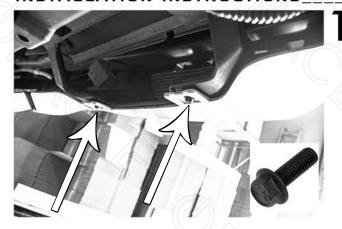
You do not need to lift the vehicle to install this product. If you decide to lift the vehicle to get better access be sure to use jack stands, wheel chocks, & proper safety protocol.
