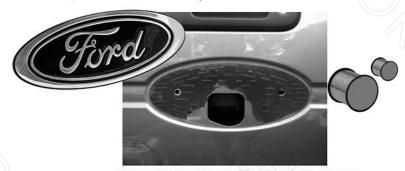
NOW USING A PIECE OF FISHING LINE, BEGIN AT ONE END OF THE EMBLEM AND WORK YOUR WAY TO THE OPPOSITE SIDE USING A BACK AND FORTH MOTION, UNTIL BADGE IS REMOVED. TO REMOVE THE EXCESS ADHESIVE, USE A TYPE OF ADHESIVE SOLVENT. MAKE SURE THE SOLVENT WILL NOT DAMAGE THE PAINT ON YOUR VEHICLE.
