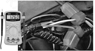
USING A MULTIMETER, TEST YOUR VEHICLE'S WIRING TO LOCATE THE PARKING LIGHT WIRING AND THE BRAKE LIGHT WIRING. TAP INTO THE PARKING LIGHT WIRING FOR CONSTANT ILLUMINATION; TAP INTO THE BRAKE LIGHT WIRING FOR ILLUMINATION WHEN BRAKING.
