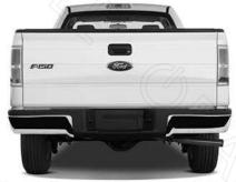
BEGIN BY REMOVING THE FACTORY BADGE. IT HELPS TO FIRST HEAT THE AREA TO SOFTEN THE FACTORY ADHESIVE. YOU CAN USE A HEAT GUN OR EVEN A HAIR DRYER.
