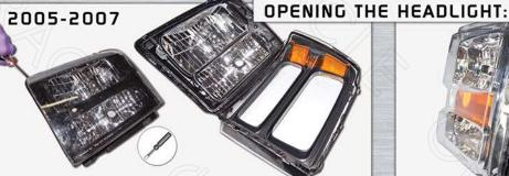
A) Start by using a flat-head screwdriver and apply pressure between the lens and housing. Caution, headlight will be hot.
