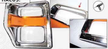
C) Drill a hole in each location marked with a red arrow. There should be (2) holes drilled. One in the corner on the bottom square and one on the flat surface in the top right. Next, remove the backing paper from the 3M adhesive and firmly press the halos into position.
