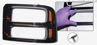
C) Drill a hole in each location marked with a red arrow. There should be (2) holes drilled. One in each corner of the housing. The wires will feed through these holes Next, remove the backing paper from the 3M adhesive and firmly press the halos into position.
