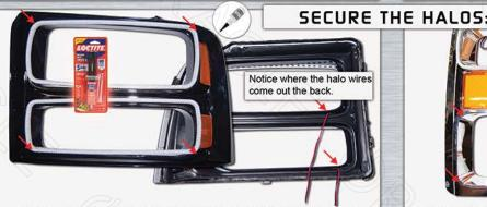
D) Use a two part epoxy or adhesive to secure the halo to the bezel edge, the locations are marked where the epoxy needs to be applied. Allow the epoxy to fully cure before moving onto the next step.
