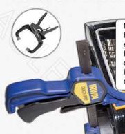
Now clamp the lens to the housing and let it sit long enough for the seal to fully set. If you used any type of sealant or silicone follow the instructions on the label for drying time.
