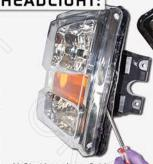
A) Start by using a flat-head screwdriver and apply pressure between the lens and housing. Caution, headlight will be hot
