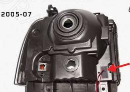
The best method to route the halo wires outside of the headlight is to make a small hole in the back of headlight venting material. Then carefully feed the wires through each hole.
