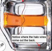
D) Use a two part epoxy or adhesive to secure the halo to the bezel edge, the locations are marked where the epoxy needs to be applied. Allow the epoxy to fully cure before moving onto the next step.
