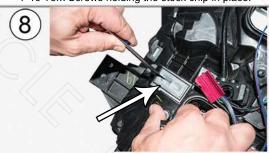
On the backside of the headlight, there is a small area of venting material. Make a small slice and route the wires out of the headlight.
