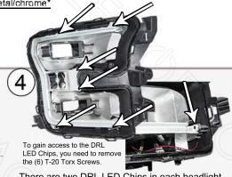
There are two DRL LED Chips in each headlight, one on each end of the clear diffuser. Once the (6) Torx Screws are removed, the white bezel can be removed as well. Disconnect the clips attaching the DRLs to the headlight.
