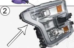
Use a flat head screwdriver to softly separate the lens and the housing.
