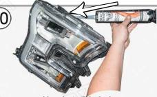
Remove any old sealant still in the lens groove. Reseal the headlight by forming a solid bead of RTV silicone adhesive We suggest using ORACLE Headlight Sealant. Allow enough time for the sealant
