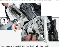
If you are are installing the halo kit, you will need to drill two small holes big enough for the wires to pass through. Remove the 3M backing and firmly place your halos to the bezel. The wires will route out the headlight just like in step 8.
