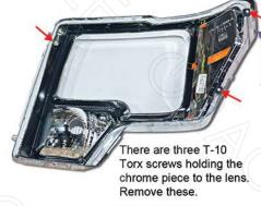
Once the chrome piece and the lens is seperated. drill a small hole here for the wires to be routed through.
