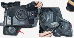
A) Start by removing this 7mm screw. Be careful the headlight will be hot.
