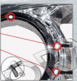
D) Next, remove the paper backing from the concept strips and install them to this piece of the chrome bezel. You may use a small amount of two-part epoxy to extra stability. The locations of where to apply the epoxy are marked below.
