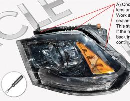
A) Once heated, begin separating the headlight lens and the headlight housing using a screwdriver. Work around the headlight prying the heated sealant until the two pieces begin to separate. This step is somewhat tedious, take your time.
