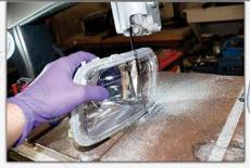
Another method to seperate the lens and housing is to use a bandsaw, if you have access to one. Remember use extreme caution and be careful.
