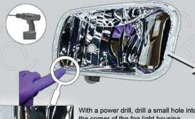
With a power drill, drill a small hole into the corner of the fog light housing. When you install your halo, you wil feed the wires through this hole first. Refer to the close up image on the
