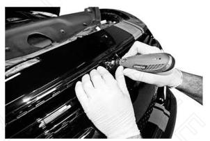
USE A DRILL TO CAREFULLY CUT A HOLE LARGE ENOUGH FOR THE WIRING TO FIT THROUGH. THE HOLE SHOULD APROXIMATELY BE 1/2" WIDE.
