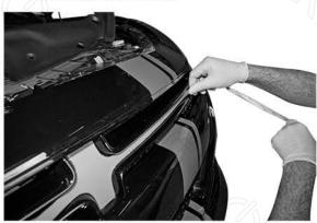
YOU ARE NOW READY TO APPLY YOUR CROSSHAIR. PREP THE SURFACE WITH AN ALOCHOL SWAB, THEN REMOVE THE 3M TAPE PROTECTIVE BACKING. START FROM THE CENTER THEN MOVE OUTWARDS.
