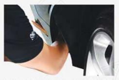
REACH INTO THE WHEEL WELL, SQUEEZE THE CLIPS ON THE BACK OF THE STOCK SIDEMARKER AND REMOVE IT
