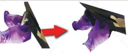
REMOVE THE STOCK SIDEMARKER FROM IT'S PLACEMENT, THEN REPLACE IT WITH YOUR NEW ORACLE LED SIDEMARKER
