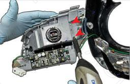
Loosen these 2 screw to seperate the reflector.
