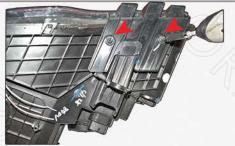
Start by using a phillips screwdriver to remove this bracket. There are 2 screws holding it in place.
