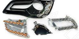
Here you can see that we have seperated all the main pieces of the headlight. Once this step is completed you can move onto the ribbon removal and install.
