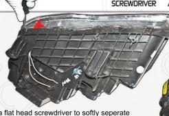
Use a flat head screwdriver to softly seperate the lens and the housing. Continue all the way around the headlight until it begins to part.
