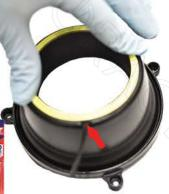
Tip: Notch out a small amount of the bezel for the wires to fit through. Makes for less of a chance of wires being bent or crimped.
