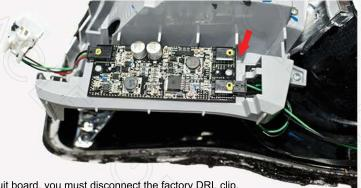
On this circuit board, you must disconnect the factory DRL clip. The new ribbon strip wire will be routed outside of the headlight. The stock clip can be removed or neatly tucked under the circuit board.
