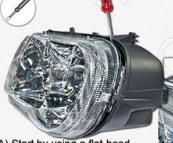
A) Start by using a flat-head screwdriver and apply pressure between the lens and housing. Caution, headlight will be hot.
