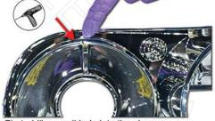
First, drill a small hole into the chrome housing. This is where you will run the halo wires through.
