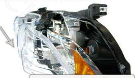
A) Begin by removing the 3M tape backing and fitting the ring to the headlight housing
