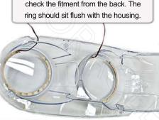
C) Optional: Use additional adhesive to hold the ring in place on the housing.
