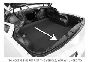
REMOVE THE REAR INTERIOR COVER PIECE. THIS PIECE IN HELD IN BY A FEW CLIPS. PULL UP ON THE COVER TO RELEASE. YOU WILL NOW HAVE ACCESS TO REAR OF THE VEHICLE.
