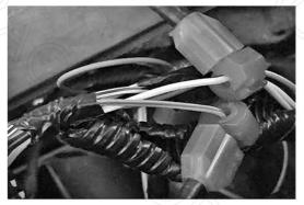
6 NOW T-TAP THE CORRECT WIRES, YELLOW/WHITE WIRE IS THE BRAKE LIGHT WIRING, THE BROWN WIRE IS THE PARKING LIGHT WIRING. IF YOU HAVE A DUAL INTENSITY EMBLEM, YOU WILL USE BOTH PARKING AND BRAKE WIRES.
