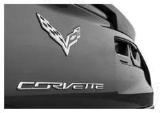
BEGIN BY REMOVING THE FACTORY BADGE. IT HELPS TO FIRST HEAT THE AREA TO SOFTEN THE FACTORY ADHESIVE. YOU CAN USE A HAIR DRYER, HEAT GUN, OR JUST PARK THE CAR IN THE SUN FOR A WHILE.
