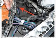
Drill a hole in the backside of the headlight for the wires to route. Be sure to seal up the hole to prevent any moisture getting inside the light.
