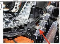
Disconnect the clip in the image above. This clip will be inserted into the RGB DRL Circuit Board.
