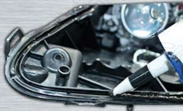
Silicone in channel close up
