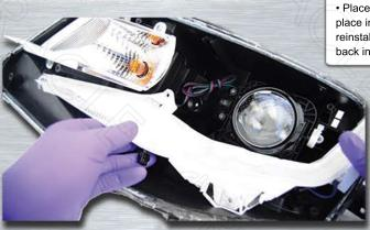
Place the Diffuser back into place inside the headlight & then reinstall the four T-25 screws back into the Diffuser
