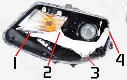
Remove the four T-25 screws from the diffuser, then carefully remove the diffuser from the housing
