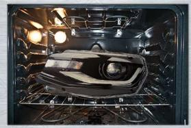
STEP #1: IN ORDER TO OPEN THE LIGHT WE WILL FIRST NEED TO HEAT THE HOUSING. IF USING A HEAT GUN BEGIN BY HEATING THE SEAL EVENLY WHILE CONSTANTLY MOVING THE HEAT GUN. IF USING AN OVEN: PREHEAT TO 225°F AND PLACE THE LIGHT IN THE OVEN FOR 10 MINUTES.
