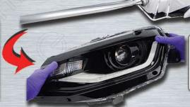
· Now place the housing back into place on the headlight & then reinstall the six T-25 screws back into the headlight
