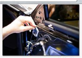
Remember to replace the rubber covers, realtach any disconnected plugs, before replacing door panel
