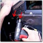
A deep socket is easier to get to these 3 bolts. If you drop the nuts inside the frame, you can remove the door speaker to retrieve them.
