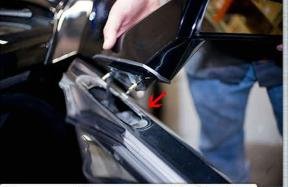
Disconnect the power plug from the stock mirror and pull the wires out. Feed the new mirror wires here.
