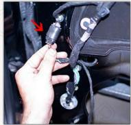
Connect the power mirror plug located here.
