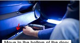
Move to the bottom of the door panel and remove the (2) 7mm bolts.
