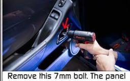
Remove this 7mm bolt. The panel is still connected to the door's harness.
