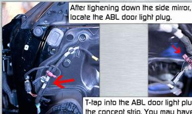
T-tap into the ABL door light plug to power the concept strip. You may have to cut some housing material to expose wires.
