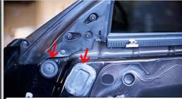
Detact the door latching wire, and any plugs still connected to the panel. Locate these rubber inserts.
