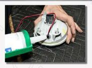
Apply a small amount of silicone to the vent hole. This is to stop moisture from building up inside your fog lights.
