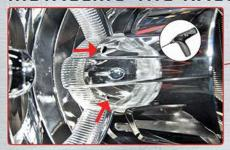
You will now drill two small holes for the halo wires to feed through.
