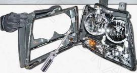
Next, use a flat head screwdriver to softly separate the lens and the housing. Continue all the way around the headlight until the lens begins to part.
