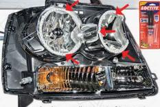
Apply a small amount of two-part epoxy to each marked spot in the above picture.
