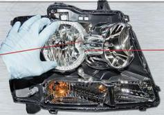
Remove the 3M backing paper and firmly press the halo to the inside of the reflector.
