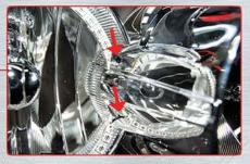
Here is a close up shot of the halo ring wires routing through the two drilled holes.
