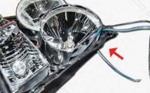
Route the halo wires from the inside to the outside before installing this halo.
