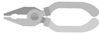
PLIERS Used to crimp t-taps. Not needed if with the P&P Adapters
