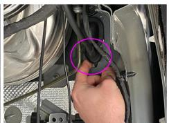
6) Route the White wire through the firewall. On the passenger side route through the main wiring harness behind the fuse box. On the Driver side route though this grommet whichis visible with the wheel liner removed (see photo).
