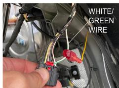
5) Now connect the turn signal (White/ Green Wire) with T-Tapand plug in the yellow wire from the Sidetrack Light. The cable is located in the fender directly above where they wires enter through the fender vent. (You can unplug for easier access but remember to plug back in).
