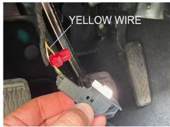
7) Now connect the Courtesy Light (Yellow/ Brown Wire) with T-Tap and plug in the White wire from the Sidetrack Light. The cable is located in the footwell and is plugged into the LED Courtesy light (You can unplug for easier access but remember to plug back in).
