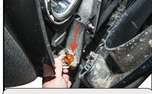
Twist and unplug the turn signal sockets from the OEM grill. Remove the turn signal bulbs.
