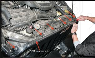
Use a flat head screwdriver or panel tool to remove the 6 clips holding the OEM grill in place.
