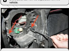
Use a 15mm Socket to remove the two headlight
