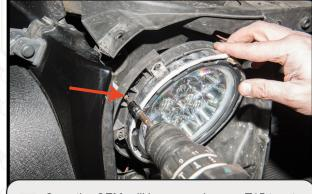
Once the OEM grill is removed, use a T15 torx to remove the headlight adjuster.
