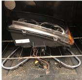
RE-INSTALL LENS TO HOUSING (PLACE IN OVEN I OM @ 235 DEGREES). CLAMP LENS AND HOUSING TOGETHER WHILE COOLING.
