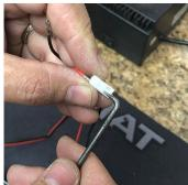
TO MAKE IT EASIER TO ROUTE THE HALO'S WIRES, USE A PICK TOOL TO DE-PIN THE HALO LED DRIVER PLUGS.
