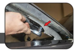
USING A 12 MM SOCKET AND SOCKET WRENCH, LOOSEN THE TWO 12 MM BOLTS.
