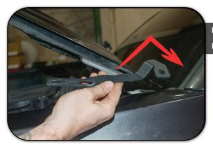
THE A PILLAR BRACKET WILL BE ORIENTED IN THIS POSITION. [SEE PHOTO] INSERTED IN BETWEEN THE HOOD HINGE BRACKET & THE HOOD.
