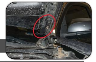
REFER TO THE IMAGE ON THE RIGHT OF THE BRACKET CORRECTLY INSTALLED. REPEAT THE PROCESS FOR THE PASSENGER SIDE BRACKET INSTALL.
