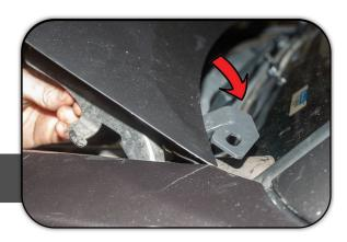
THIS PORTION OF THE BRACKET WILL PASS UNDER THE BOTTOM AND AROUND THE TOP OF THE HOOD.
