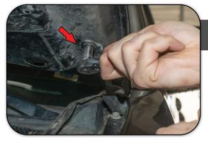
POP THE HOOD AND LOCATE THE TWO 12MM BOLTS ATTACHING THE HOOD HINGE BRACKET TO THE HOOD.
