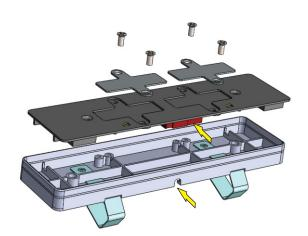
Use the components removed from the original Trigger base to assemble the Visor mount as shown. Note the location of the 12 volt power connector and slot for the 12 volt wiring as indicated by the arrows.
