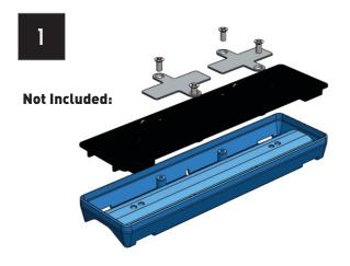
Begin assembly by removing the inner plate of the original Trigger mount included with the Trigger 6 Shooter kit. Remove the four screws and set aside with the top plate/wire/connector, all will be re-used for the visor mount.
