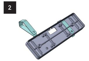
Insert the metal visor clips into the base as shown, be sure they go all the way in and snap over the raised round detail.
