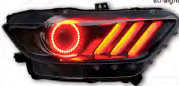
RGB 5050 Concept SMD strips installed as Daytime Running Lights behind the OEM diffusers.
