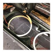
ONCE EPOXY DRIES, REMOVE TAPE AND PAPER COVERING THE 3M ADHESIVE BACKING.
