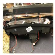
ROUTE WIRES THROUGH HEADLIGHT BASE VENT HOLES AS SHOWN, THEN RE-PIN LED DRIVER PLUGS.
