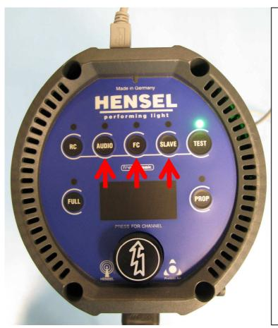
Press the three with red arrows marked push-buttons with switched off Expert D unit and then switches the unit on. The green ready LED lights up. Programming mode of the Expert D is now active. If for the first time an Expert D is stuck on to a computer, you receive the message at the computer "the new hardware was found ". Please wait until the new hardware is installed.
