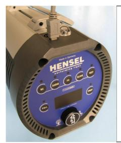
Connect the unit by the USB socket with the computer before switching on.
