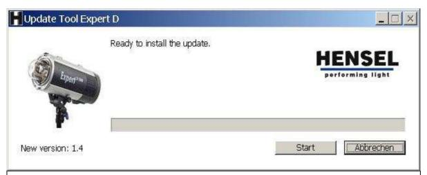
If the equipment were attached correctly, the above window appears. For programming click on the button "start". While programming runs, do not switch off the computer or separate the equipment!
