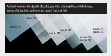
Code No. 726 // HEAVY FROST, diffuser foil, very matt, available by the meter, 1.22 m wide Code No. 736 // HEAVY FROST, diffuser foil, very matt; roll 1.22 W x 7.6 m L
