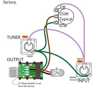
A better idea is to use an external pedal power supply. Then you can leave the output jack plugged in and not worry about battery life. ALSO, the Redeemer Ai1 can take up to 36V for maximum headroom. I would want at least enough headroom to handle the loudest pedal in my chain... so, if I had an 18V pedal, I would use at least 18V to power the Ai1 too. J3 "Sleep Enable" could be cut, however, in this case it really doesn't matter.
