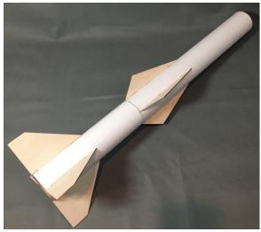
☐ Using a pencil and a straight edge, mark a line in between two of the fins the length of the tube. Epoxy one lunch lug even with the aft end of the tube. Make a mark 2" from the forward end of the tube on the same line. Epoxy the other launch lug aft of the 2" mark. Fillet the lugs for added strength.
