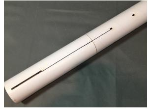
☐ Using epoxy, apply a band of epoxy inside the main airframe tube about 1-3" from the aft end. Insert the tube into the lower tube assembly all the way in until two tubes meet. Make sure the alignment lines match.
