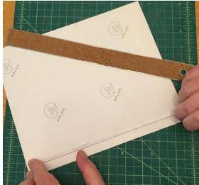
□ On a clean work surface, position the wrap on the tube. The wrap is sized to be ever so slightly longer than the 10" body tube. After the wrap is applied, the upper edge off is trimmed off. To position the wrap, begin by sitting the tube upright on the table and starting to position the wrap with the bottom edge also flat on the table. Note that nothing is being stuck to the tube at this point.
