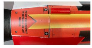
$\hfill \Box$  Using epoxy, glue the fins in place on the lower body tube. Alternate red and white fins.
