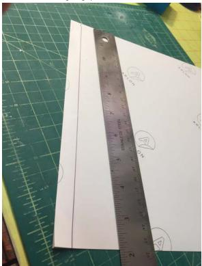
□ Now you want to fold back the backing paper along the line you've drawn. The plan is to tear off that piece of backing paper and then stick it back down into place. So don't worry, there is no preciseness necessary for this step. The next several photos show how to fold the paper back. Try to be careful not to let stuff fall onto the exposed sticky back of the wrap.
