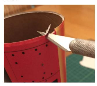
☐ Remove the wrapping covering the Launch Lug positions. Use your sharp knife to incise all four edges of each Launch Lug location. Once all four edges are cut, slip the knife point under one edge and gently lift the covering piece away.
