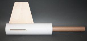
☐ Locate one of the couplers; mark it at half it's length. Test fit it in the slotted tube assembly. Using epoxy, bond the coupler in place.
