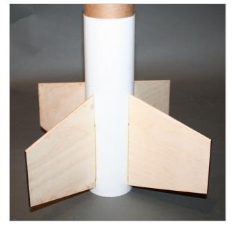
☐ Using a pencil and a straight edge, extend a 2" line in between two of the fins on the lower body. Locate the other launch lug and epoxy it in place. Fillet the lug for added strength.
