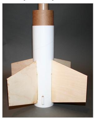
☐ Locate the remaining coupler; mark it at half it's length. Test fit it in the payload section. Using epoxy, bond the coupler in place.
