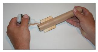
□ Locate the one of the aft/mid centering ring (one with the four slots in it) and slide it onto the motor tube to mate with the key. Using epoxy, bond the ring in place. Repeat with the other ring in the mid location.
