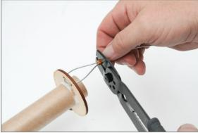
□ Place the other loop/sleeve connector on the free end of the cable. Slide both of the heat shrink sections onto the cable. Make a 1-2" diameter loop and thread the free end back through the loop/sleeve connector. Crimp the loop/sleeve connector with a crimping tool or a pair of pliers. Apply a drop of CA to the connector.
