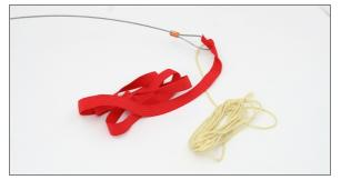
□ Coil up both the aramid and elastic shock lines and stuff them into the forward end of the motor tube. This will keep them out of the way when then motor mount is bonded in place.
