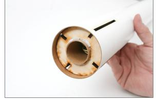
□ Using epoxy, glue the fins in place on the lower body tub
