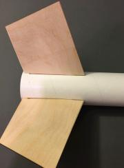
□ Locate the coupler; mark it at half it's length. Test fit it in the aft fin section. Using epoxy, bond the coupler in place.
