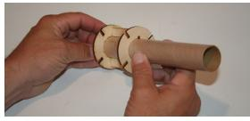
□ Locate the forward centering ring (the one with the two holes in it) and slide it onto the motor tube to one of the 1" marks. Using epoxy, bond the ring in place.
