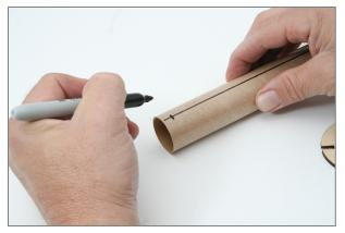
□ Mark the motor tube 1" from each end, and extend those lines around the circumference of the tube.
