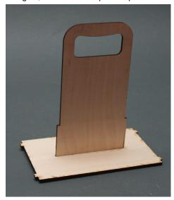
☐ Test fit the top plate through the center handle. Sand as necessary to ensure a good fit. Using CA or wood glue, bond the top plate in place.
