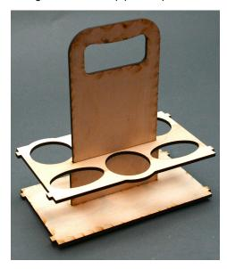
☐ Test fit one side plate on to the tabs of the base and top plates. Sand as necessary to ensure a good fit. Using CA or wood glue, bond the plate on to the assembly. Repeat for the other side.
