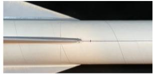
☐ Using the conduit cutting guide, mark each of the two balsa conduits as shown. Cut away the top part of the balsa stick.
