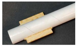
□ Locate one of the aft/mid centering rings (one with the four slots in it) and slide it onto the motor tube to mate with the key. Using epoxy, bond the ring in place. Repeat with the other ring in the mid location. Fillet both rings to the tube. Set aside to cure.
