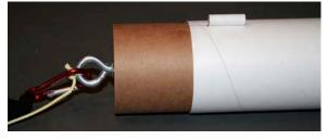
☐ Using a pencil and a straight edge, extend a line the full length of one main tube 1/2" above the fin. Repeat for the fin 180 degrees opposite the first one. This is where the conduits will go.
