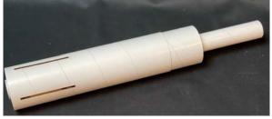
☐ Locate the forward centering ring (the one with the two holes in it) and slide it onto the motor tube to one of the 1" marks. Using epoxy, bond the ring in place. Set aside to cure.
