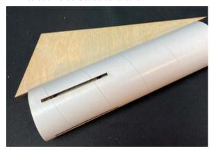
☐ Locate the white coupler; mark it at half it's length. Test fit it in the slotted tube assembly up to the mark. Remove the coupler, and apply epoxy to the inside of the tube, and re-insert the coupler up to the mark. Set aside to cure.
