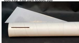
☐ Using a pencil and a straight edge, extend a 2" line in between two of the fins on the lower body. Make another mark 1/8" from the end of the tube. Locate one launch lug and epoxy it in place. Fillet the lug for added strength.
