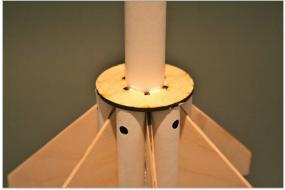
□ Locate the forward centering ring (the one with the two holes in it) and slide it onto the motor tube at the forward 0.25" mark. Using epoxy, bond the ring in place.
