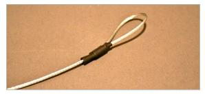
☐ Tie one end of the aramid shock line onto the top cable loop and triple knot it. Secure the knot with a drop of CA. Trim the excess off.
