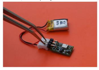
When you reset the altimeter with the manual method, you do not erase the pervious data on the altimeter. When the altimeter detects launch and begins measurement (indicated by two blinks) the previous data is deleted.
