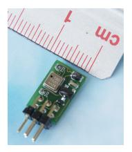
The altimeter height measurement is based on the change of pressure as a function of altitude. The altimeter pressure sensor, calibrated at the factory, measures absolute pressure.
