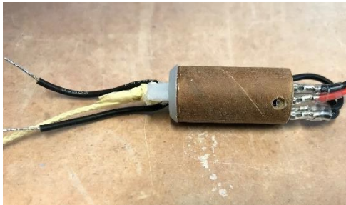
Altimeter inside 13mm coupler Battery placed above in body tube
